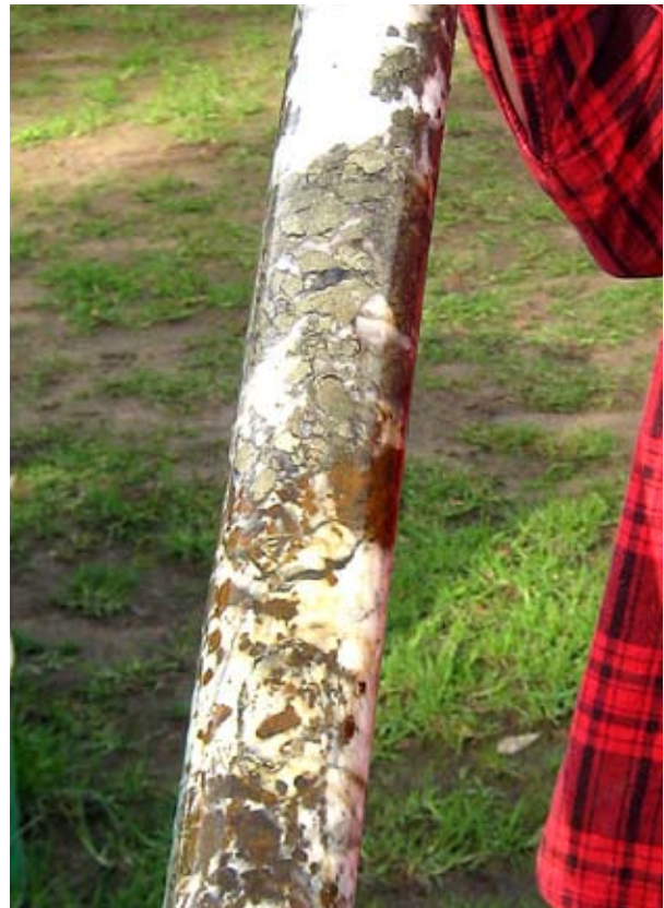
Figure 3 Core from BH 30 showing mineralised zone.
