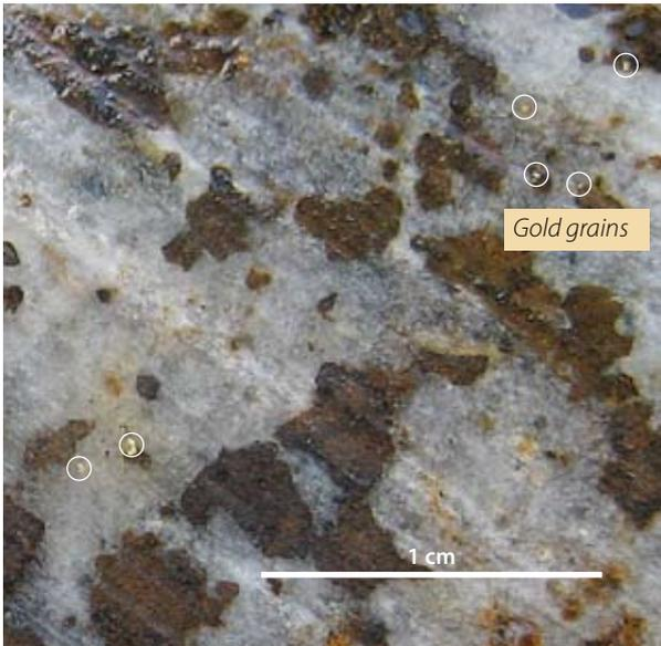
**Figure 3** Core from BH 32 showing visible grains of gold.
