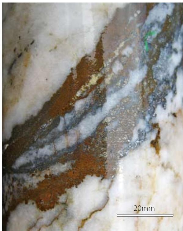
**Figure 2** Example of pyrite, limonite and galena mineralisation in drill core (BH 40).
