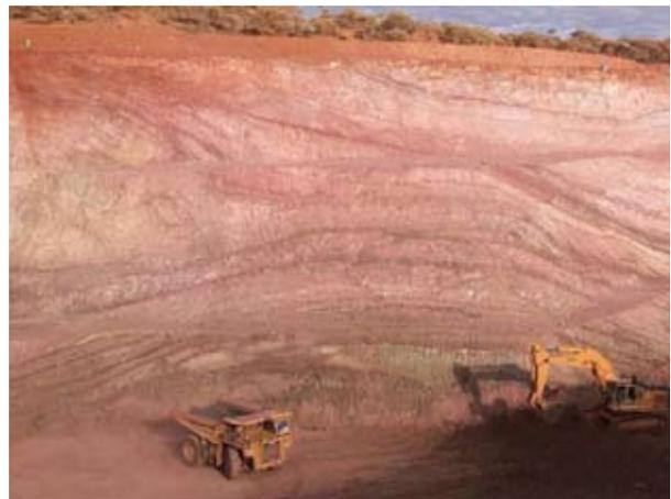
Figure 2 Precious Metals Australia's Windimurra Vanadium open cut mine (dark bands in wall of pit are massive magnetite). Photo courtesy of PMA.
