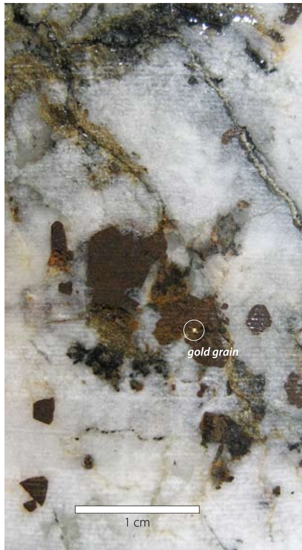
Figure 2 Core from drill hole BH 41 showing visible gold grain
