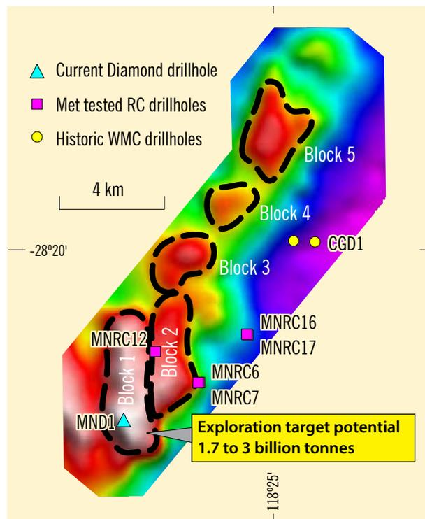
**Figure 3** Current diamond drillhole and previous drilling, shown on a gravity image of the Canegrass Magnetic Zone.
