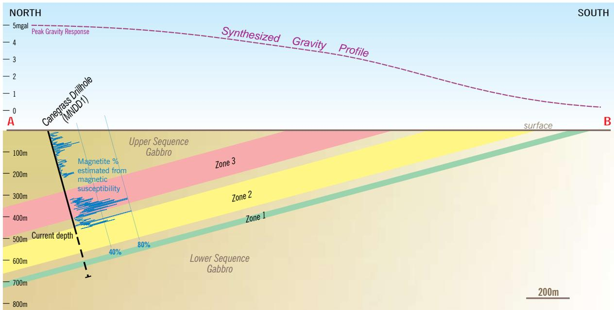
Figure 7 Current diamond drillhole in progress showing magnetic susceptibility readings on geological cross section A-B.
