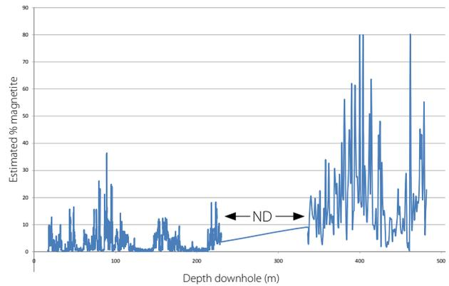
**Figure 5** Magnetic susceptibility readings on core converted to % magnetite content. (ND - no data currently available)
