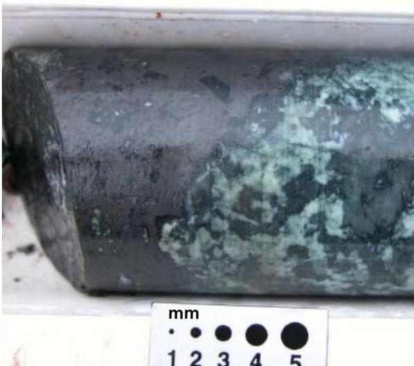
**Figure 4B** MND1: Depth 506.25m – 90% magnetite adjacent to very coarse-grained magnetite gabbro.
