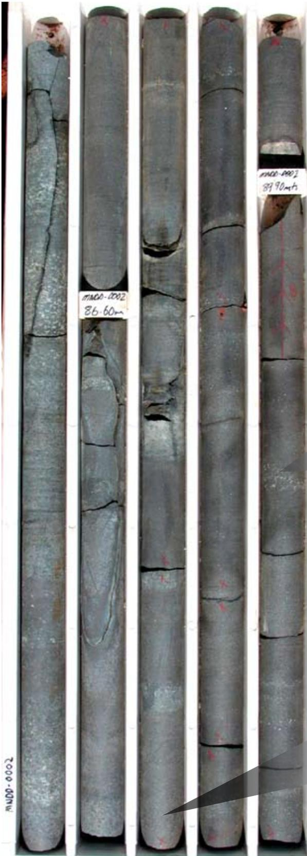
**Figure 2A** Diamond drill core tray of magnetite-rich gabbro from 85 to 90 metres depth in hole MND2. The visual average estimate is 40–55 volume % magnetite which equates to about 62 weight %. Figures 2B and 2C are close ups on sections of drill core showing dark grey magnetite with magnetic susceptibility readings (k values) indicated.
