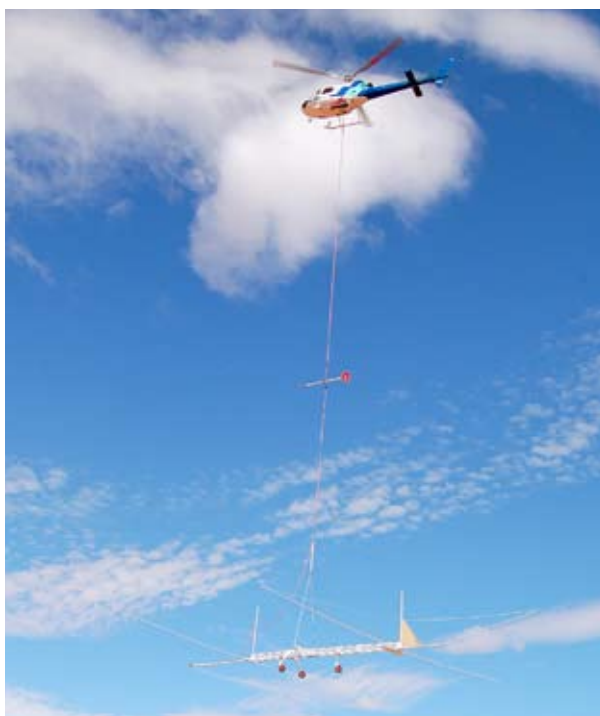
Figure 1 REPTM system in operation, showing EM loop below and magnetometer between loop and helicopter.
