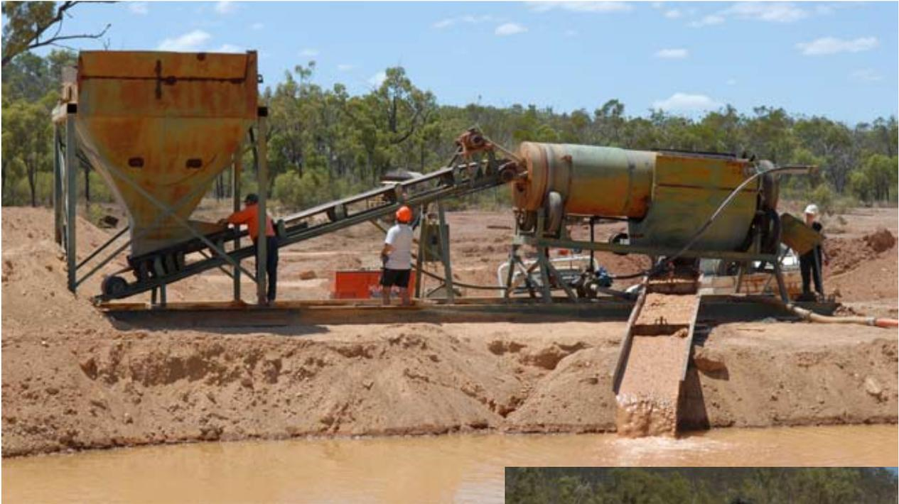
**Figure 2** The refurbished scrubber-trommel plant operating at Sellheim.
