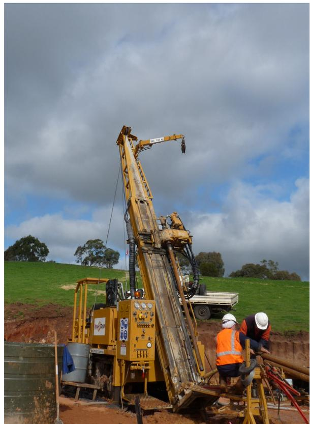
**Figure 1** Diamond drilling at Deloraine.
