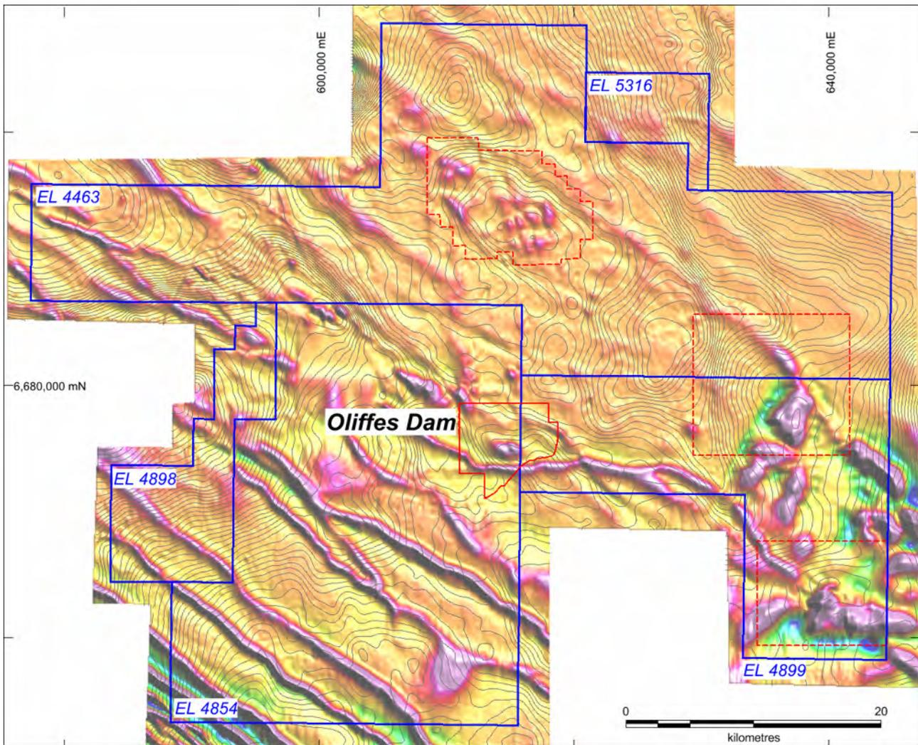
**Figure 2. Background reduced to pole (RTP) magnetic image for Millers Creek DP, further processed with a high pass filter, highlighting shorter wavelength features. 2013 WPA gravity survey data merged with open file gravity data with old pre 1970 data deleted is shown as contours (5gu/0.5 Mgal contours).**
