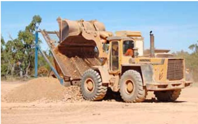
Screening Golden Triangle oversize prior to trucking to trommel plant.
